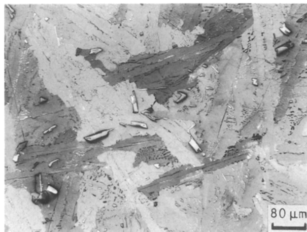
Figure 3 Optical micrograph of a 3:1:2 sample quenched from 820 °C (slightly uncrossed polars). The quasi-eutectic microstructure is formed by the \beta -phase which includes fine directed CuO precipitations and larger, partly dissolved CuO grains.
